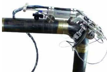
PET applied to a 4" pipe bend
