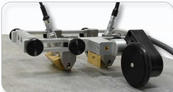
Weld inspection using WREN 4 with 60° brass wedges
