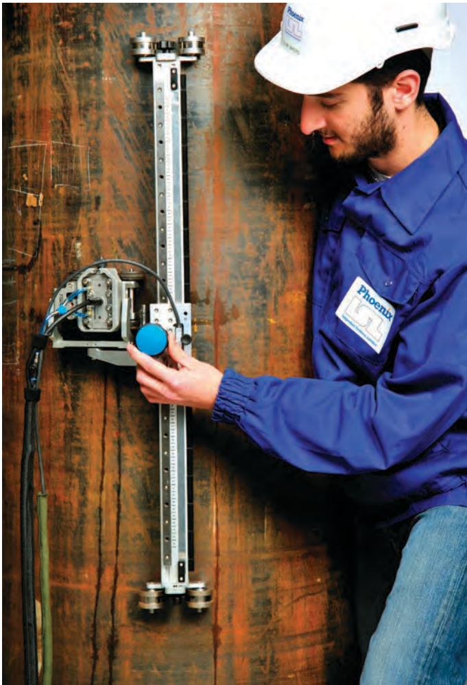
MapMan performing corrosion scans on 24" OD pipe
