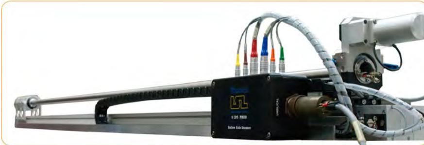
Originally designed for the rail industry for the inspection of train axle bores, this scanner can be adapted for any type of bore inspection and is
